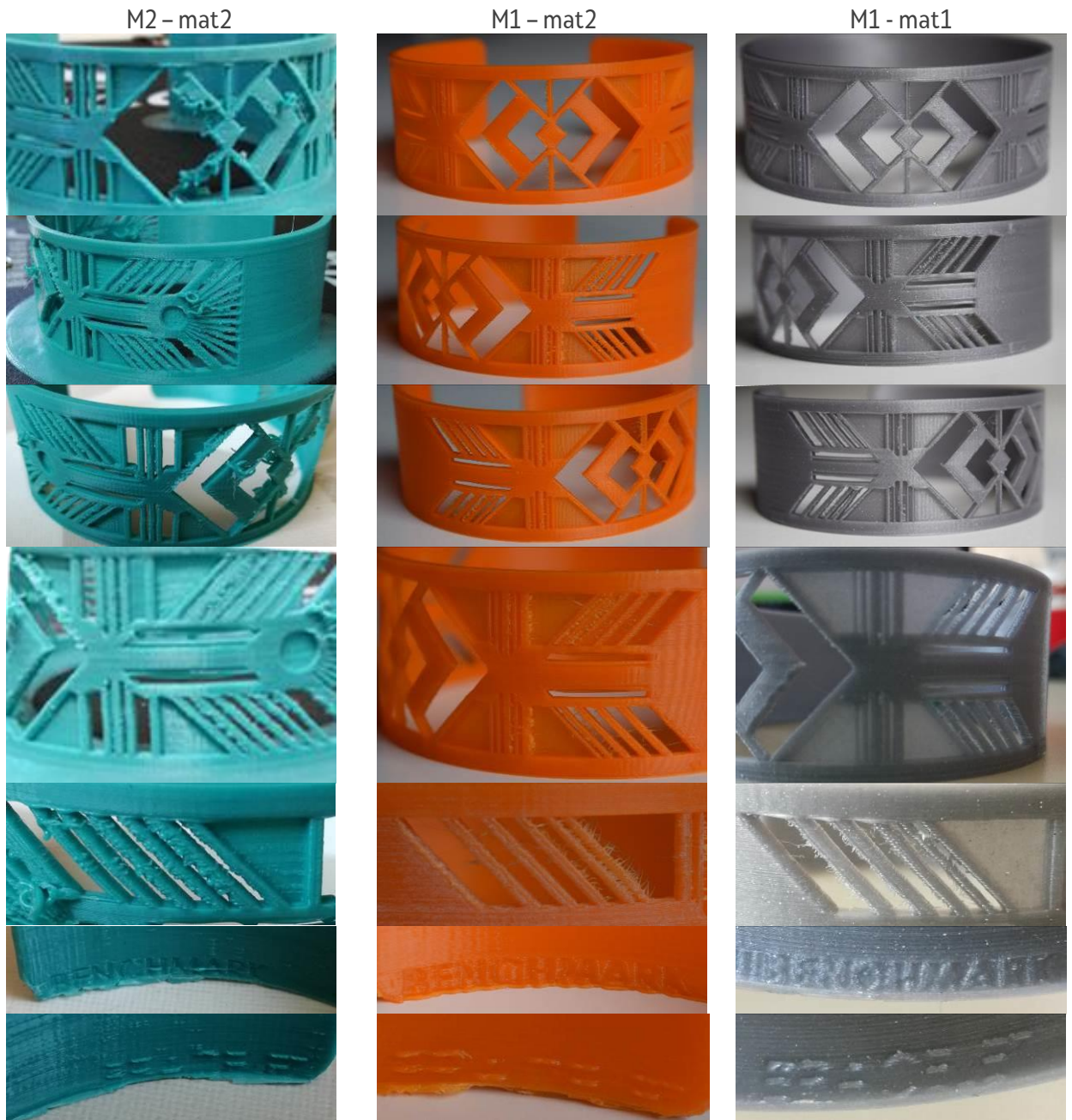
Figure 5-1. Comparison of details of the BM fabricated on different FDM machines with same parameters (personal research)
